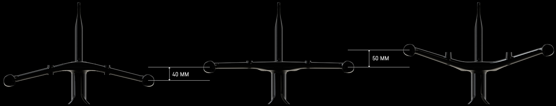
DROPPED BASEBAR POSSIBLE TO MOUNT EXTENSIONS BELOW BASEBAR
