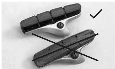
Brake pads with worn down wear indicators, i.e. grooves, (bottom brake pad) must be replaced by original spare parts
