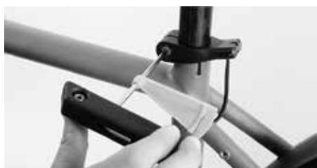
Tighten the locknut by using the Canyon torque wrench according to the torque values on the Wheelguard
