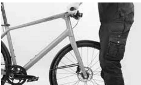
Try twisting the handlebars relative to the front wheel
