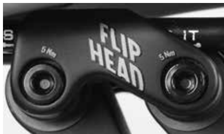
Do not exceed the indicated maximum torque value!
