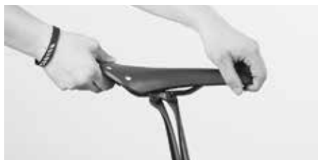
Try twisting the saddle relative to the frame
