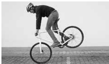
Too hard braking with front brake; do not imitate
