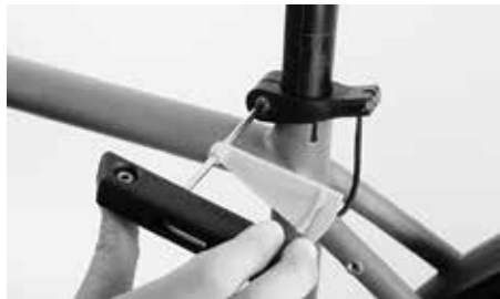
Mounting the seat post with the Canyon torque wrench
