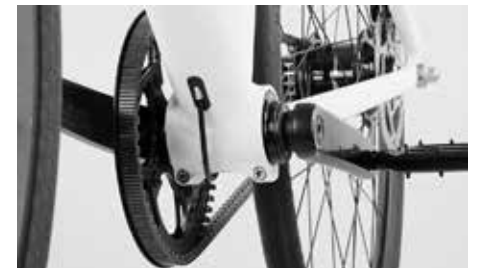
Check the proper fit of the eccentric bearing in the BB shell
