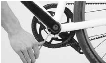
Turning the eccentric bearing, increasing tension
