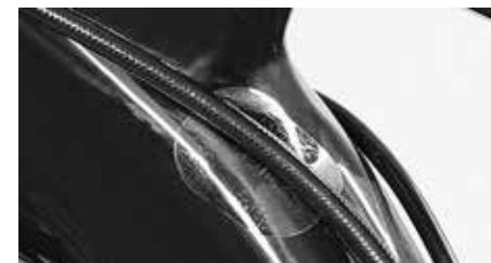
Special pads protect carbon from damage
