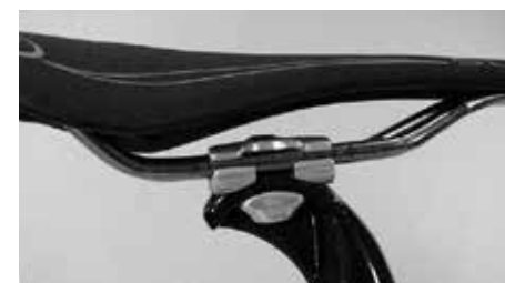
Be sure the saddle rail is clamped within the marked area
