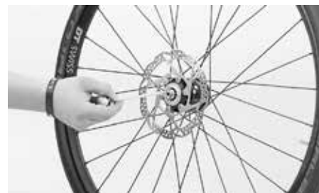
Slide Wheelguard into the hollow axle
