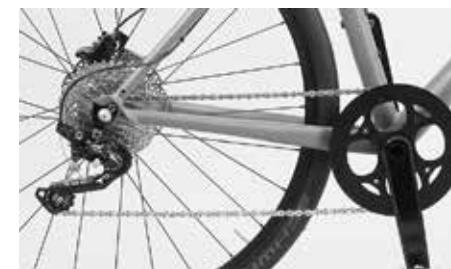
Store the bike with the chain on outmost sprocket and smallest chainring
