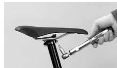
Retighten the bolts evenly and alternately to the prescribed torque value
