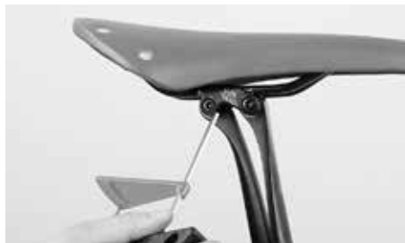
Tighten both bolts evenly and alternately without exceeding the permissible maximum torque value
