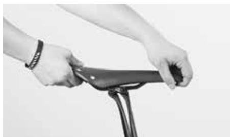
Check the firm seat of the retightened saddle
