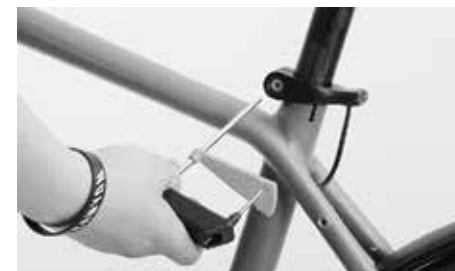
To adjust the saddle height release the Wheelguard at the seat post binder bolt
