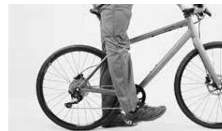
The leg must be fully stretched with the heel on the pedal at its lowest point
