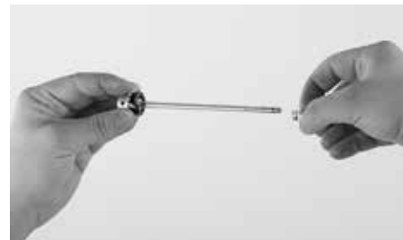
Remove locknut and spring from the Wheelguard
