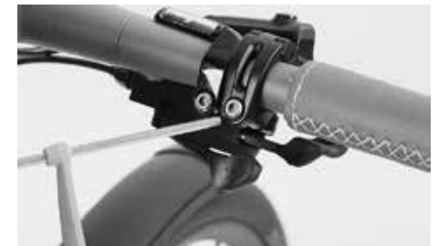
Tighten the brake and shift lever mounts to the prescribed torque values
