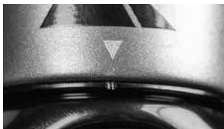
Correct alignment of IPU – arrow and groove on top of one another
