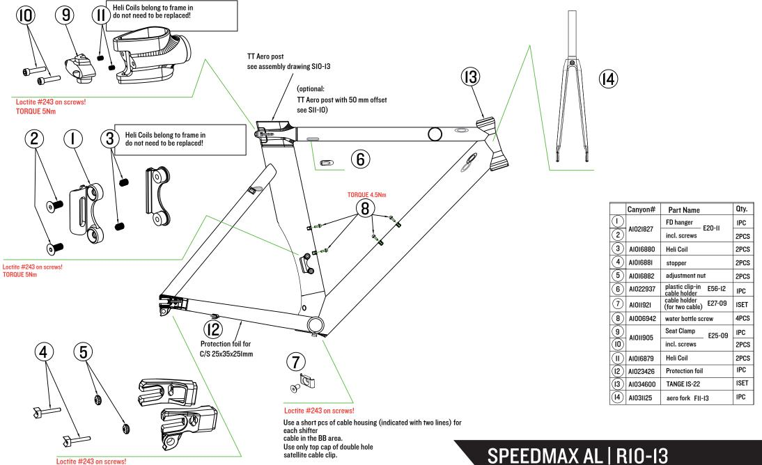
Note: Part 4 is assymetrical! Make it flush on inside and outside. SPEEDMAX AL | RIO-I3
