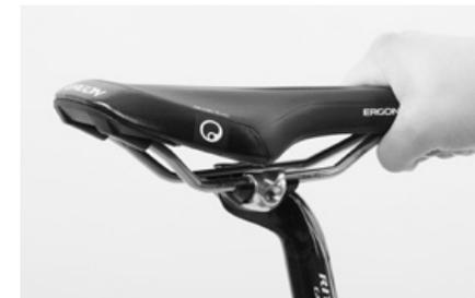
Bring the saddle into alignment and do not overtighten the quick-release or the seat post binder bolt, i.e. do not exceed the permissible maximum torque. Use the Canyon Torque Wrench.
