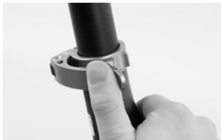
Slide the seat post into the seat tube to the desired minimum saddle height. Please note the MIN/MAX marking on the seat tube. Bring the saddle into alignment and close the quick-release or the seat post binder bolt. Take care not to overtighten the seat post binder bolt or quick-release.
