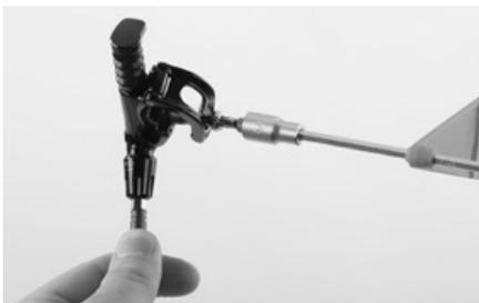
Take the matching bit from the Toolcase and release the Torx screw from the control lever.
