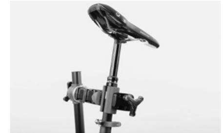
**i** Do not clamp a frame tube or a carbon seat post of your Canyon in the holding jaws of the workstand! Use a suitable aluminium seat post for clamping instead. If you have a height-adjustable seat post, do not clamp the bike on a movable part, but only on the bottom part which is removed far enough. When inserting or pulling out the height-adjustable seat post, make sure to pull in or out the cable where it comes out of the frame to prevent any breaking of the cable.
