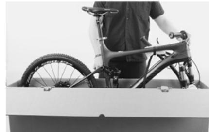
Lift the frame carefully off the BikeGuard and make sure it stands safe.
