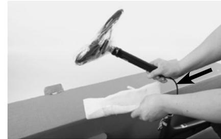
If your Canyon has a height-adjustable seat post, mount the height-adjustable seat post before lifting the Canyon out of the BikeGuard. The height-adjustable seat post is ready-for-use connected by means of a cable running through the seat tube with the control lever mounted at the handlebars.
