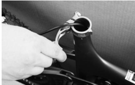
You should be able to insert the seat post easily into the frame without pressing or turning. If you are not, loosen the seat post binder bolt a little more.
