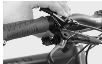
Remove the protective film from the right brake lever.
