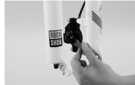
Remove the protective film from the fork, if available. It is recommended that you remove the protective material in general by hand. If that is not possible, it is best to use scissors. Do not use a box cutter. Remove the transport locks from the front wheel brake. For more information about brakes, read chapter "The brake system" in your bicycle manual Mountain bike; also observe the instructions of the component manufacturers on the enclosed CD.
