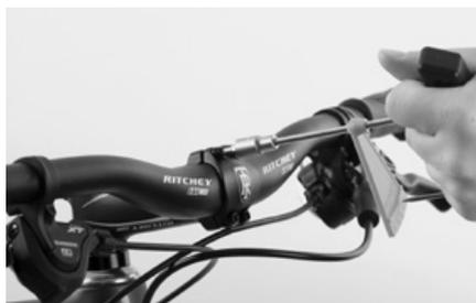
Position the faceplate on the handlebars. Retighten the clamping bolts of the faceplate evenly in a cross pattern until they lightly hold the handlebars in place. Bring the handlebars roughly into the adequate position so that the brake levers slightly point downwards.
