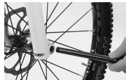
If your bike is equipped with a Maxle thru axle system with quick-release lever, put the front wheel into the fork and mount the rotor in the brake calliper.
