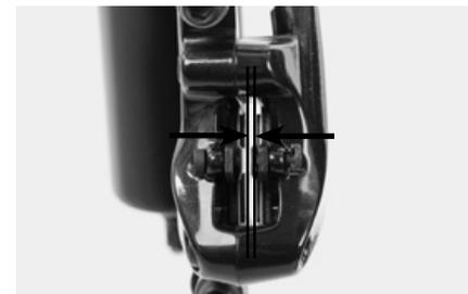
If your Canyon has disc brakes, check before mounting the wheel whether the brake pads rest snugly in their seats in the brake calliper body. This is the case when the gap between the brake pads is parallel.
