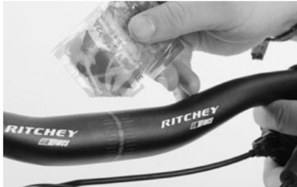
Prior to applying Canyon assembly paste, remove dirt particles and lubricant residues from the surfaces to be treated. Apply a thin and even film of Canyon assembly paste to the cleaned surfaces using a brush or a chamois.
