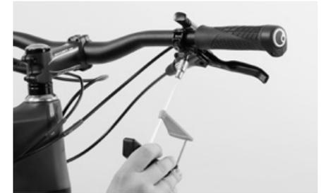
Tighten the bolt to the tightening torque of 5-6 Nm specified by SRAM.
