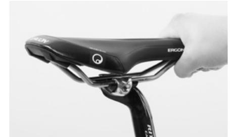
Bring the saddle into alignment and do not overtighten the quick-release or the seat post binder bolt, i.e. do not exceed the permissible maximum torque. Use the Canyon Torque Wrench.
