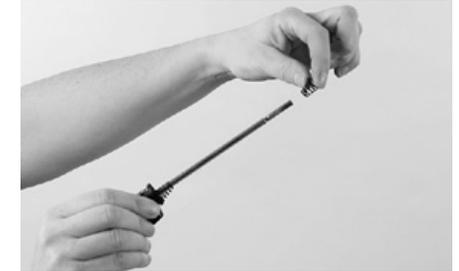
Take the quick-release for the front wheel out of the small parts box. Release the counter-nut and remove one of the springs from the quick-release.
