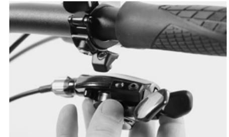
Assemble the shift lever to the Matchmaker. Tighten the bolt to the tightening torque of 2.8-3.4 Nm specified by SRAM.
