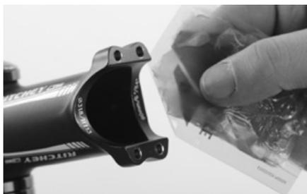
Squeeze out some Canyon assembly paste and apply a thin layer of carbon assembly paste on the inner side of the faceplate as well as in the clamping area of the stem body.
