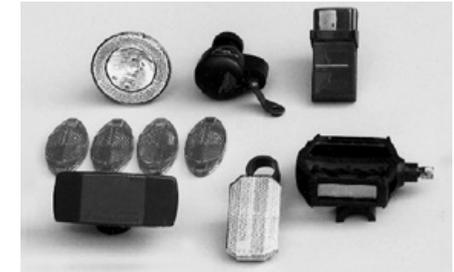
Fix the white reflector to the handlebars and the red reflector to the seat post as well as a bell.
