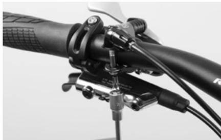
Now you can tighten the bolt of the control lever with the Canyon Torque Wrench.
