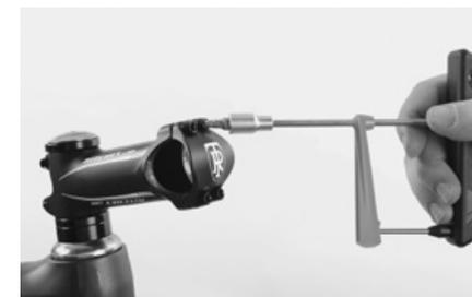
Take the Canyon Torque Wrench and put the bit matching the faceplate bolts into the holder.
