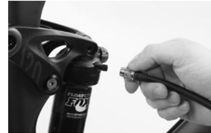
Inflate the rear shock with the special pump enclosed with the BikeGuard, according to the recommendations of the rear shock manufacturer. You will find the operating instructions of the rear shock manufacturers on the enclosed CD.
