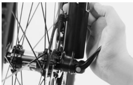
Close the E-Thru quick-release lever like a usual quick-release lever. From the start of the closing movement up to about the first half of its travel the lever should move very easily without clamping the wheel, whereas over the second half of its travel the force you need to move it should increase considerably. Towards the end of its travel the lever should be very hard to move.
