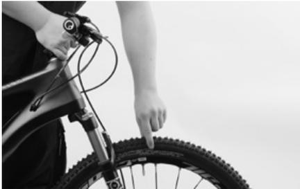
After mounting the wheel and tightening the quick-release or the thru axle pull the brake lever several times and spin the wheel subsequently.
