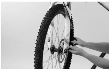
Mount the front wheel and make sure you guide the rotor between the brake pads carefully. Close the quick-release and verify that the wheel is securely fixed. Read the chapter “How to use quick-releases and thru axles” in your bicycle manual Mountain bike beforehand.
