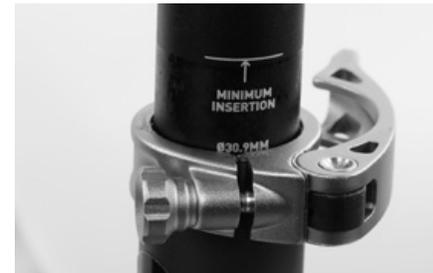
Your seat post must go into the frame as a minimum to as far as underneath the top tube and up to the MIN/MAX marking of the seat post.
