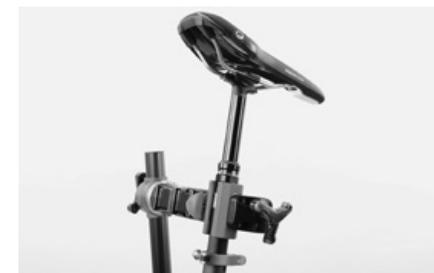
**i** Do not clamp a frame tube or a carbon seat post of your Canyon in the holding jaws of the workstand! Use a suitable aluminium seat post for clamping instead. If you have a height-adjustable seat post, do not clamp the bike on a movable part, but only on the bottom part which is removed far enough. When inserting or pulling out the height-adjustable seat post, make sure to pull in or out the cable where it comes out of the frame to prevent any breaking of the cable.
