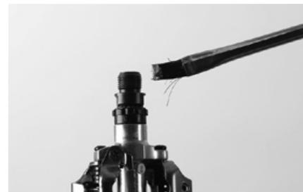
Apply a thin layer of standard assembly grease on the pedal threads before screwing in the pedals.
