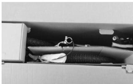
The BikeGuard contains the assembled frameset with the rear wheel mounted and all add-on parts as well as the front wheel that is sometimes packed in a wheel bag, the saddle with seat post, which may be connected with a cable to a control unit to be mounted on the handlebars.
