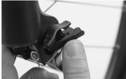
As soon as the axle thread engages with the thread of the left fork leg, close it by turning it clockwise. During the first rotations you should be able to rotate the thru axle nearly without resistance. Tighten the axle until it is hand-tight. Re-fold the lever of the thru axle.
