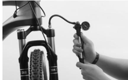
Inflate the suspension fork with the special pump enclosed with the BikeGuard, according to the recommendations on the spring rate of the fork manufacturer. You will find the operating instructions of the suspension fork manufacturers on the enclosed CD.
