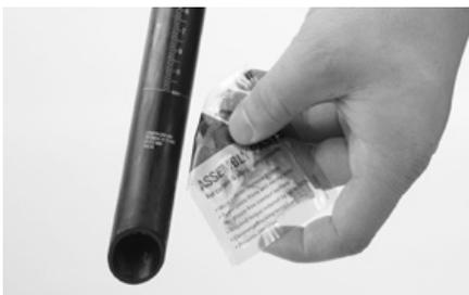
Apply a little Canyon assembly paste to the bottom part of the seat post and inside the seat tube or in the clamping area of the seat post.
