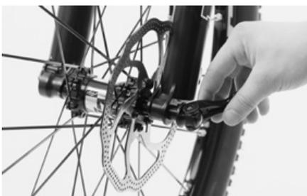
As soon as the axle thread engages with the thread of the right fork leg, close it by turning it clockwise. During the first rotations you should be able to rotate the thru axle nearly without resistance. Tighten the axle a little and then release it by about a third of a turn.
