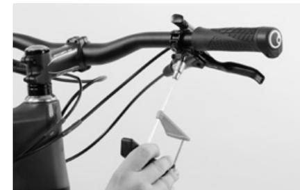
Tighten the bolt to the tightening torque of 5-6 Nm specified by SRAM.
