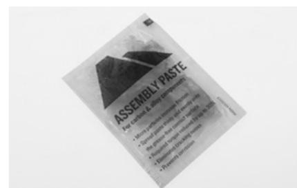
Carbon fibre components are particularly vulnerable to damage caused by excessive clamping force. Canyon assembly paste creates extra friction between two surfaces, allowing the necessary torque value to be reduced by up to 30%.
