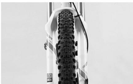
Make sure the front wheel is accurately centred between the fork blades. Make sure the quick-release lever and the drop-out safety-tabs are properly closed.
