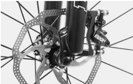
The rotor must not drag heavily on the brake calliper and normally not on the brake pads. Spin both wheels to make sure they run true.
