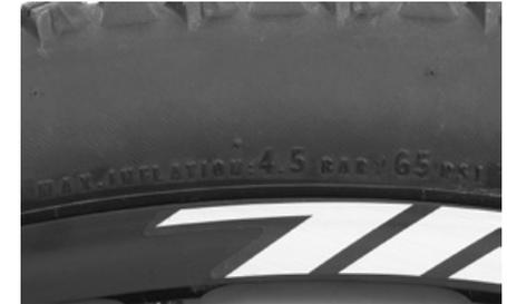
Inflate both tyres to the maximum pressure indicated on the side of the tyres. You can find more information on tyres and inner tubes in chapter **“The wheels - tyres, inner tubes and air pressure”** in your bicycle manual Mountain bike on the enclosed CD.
