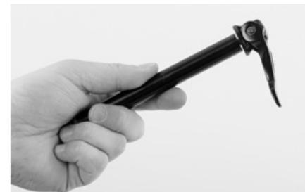
Take the thru axle for the front wheel out of the small parts box.
