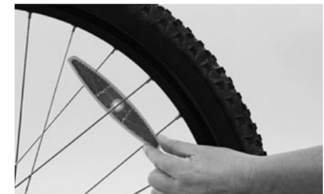
Finish by mounting the spoke reflectors. Make sure you mount two reflectors opposite of each other to the spokes of the front wheel and two reflectors opposite of each other to the spokes of the rear wheel.
