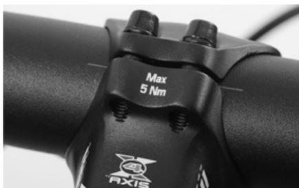
Exceeding the maximum torque at the clamping bolts (e.g. at the stem, seat post or seat post clamp) leads to an excessively high clamping force. This can cause the component to fail and hence there is a high associated risk of accidents. In addition, the product guarantee would be null and void in such a case. Screws or bolts that are too loose or are done up too tightly can cause a failure and hence lead to an accident. Always follow exactly the tightening torque details from Canyon.
