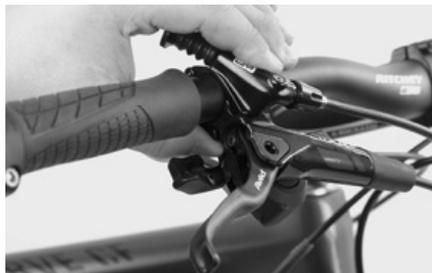
The shift lever is mounted to the handlebars, the brake lever however not.
