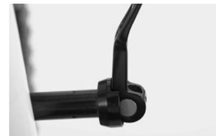
Make sure the quick-release lever is completely open and lies in the axle recess. As soon as the axle thread engages with the thread of the left fork leg, close the axle by turning it clockwise. During the first rotations you should be able to rotate the thru axle nearly without resistance.
