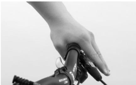
Make the adjustments of the handlebars with the front wheel mounted and the tyre inflated to the suitable pressure. The brake levers of a ready-for-use mountain bike point slightly downwards. When you sit in the saddle with your fingers on the brake levers the back of your hands should form a straight line with your forearms.
