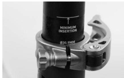
Slide the seat post into the seat tube to the desired minimum saddle height. Please note the MIN/MAX marking on the seat tube.
