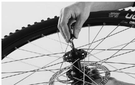
Tighten the conternut of the quick-release by no more than two full turns. Read up on quick-releases in chapter “How to use the quick-releases and thru axles” in your bicycle manual Mountain bike; also observe the instructions of the component manufacturers on the enclosed CD.
