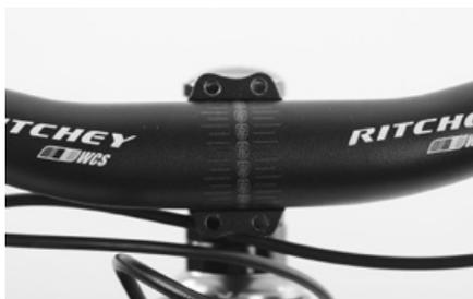
Position the handlebars by means of the marking accurately centred in the stem clamp. Make sure the bowden cables and the lines are not twisted or bent, but run in a smooth curve to the cable stops or brakes.
