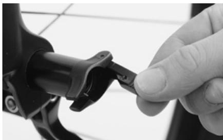
Bring the front wheel into the right position between the drop-outs and slide the axle from the right side through the drop-out and the hub. Unfold the lever from the axle.
