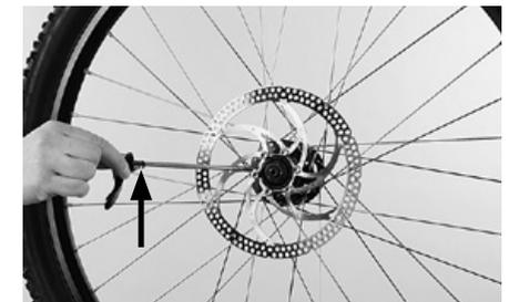
Insert the quick-release into the hollow front wheel axle.
