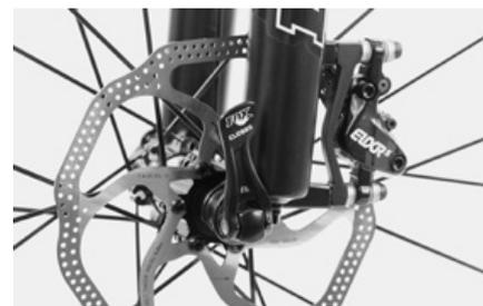
In its end position the quick-release lever should be tight so that it can no longer be turned. Make sure the quick-release lever does not stand out to the front or to the side. The best closing position is in nearly upright position in front of the lower leg.
