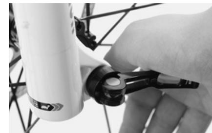
Now turn the lever forcefully clockwise until the axle is hand-tight. Make sure the quick-release lever does not slip out of the axle recess during tightening.
