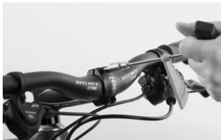
Use the Canyon Torque Wrench and finish by tightening the clamping bolts in cross pattern. Do not exceed the maximum tightening torques mainly printed on the stem!
