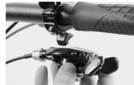
Assemble the shift lever to the Matchmaker. Tighten the bolt to the tightening torque of 2.8-3.4 Nm specified by SRAM.
