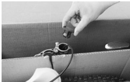
Remove the protective cap from the top end of the seat tube.
