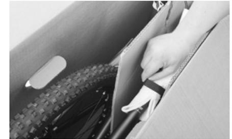
Undo the band with Velcro fastener fixing the saddle and the seat post to the front wheel.
