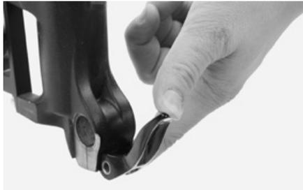
The 20-mm thru axle system provides several appliances to fix the front wheel. To mount the front wheel open both quick-release levers in the bottom area of both fork legs. Put the front wheel into the fork and mount the rotor at the same time in the brake calliper.
