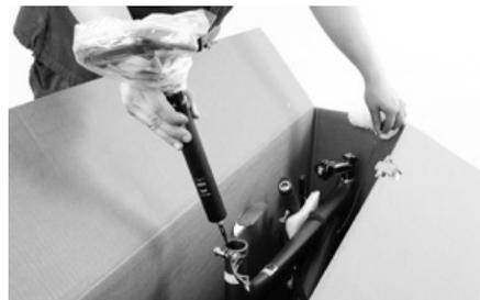
Keep the seat post in one hand and take hold of the seat post cable where it comes out of the frame. While carefully inserting the seat post with one hand into the seat tube, pull out the cable with the other hand.
