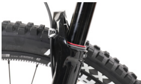
Slip a cable binder over the stanchion tube
