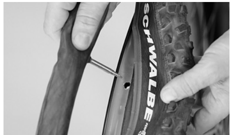
Put the valve into the rim hole
