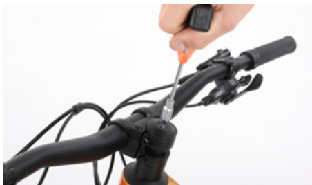
Readjust the bearing and retighten the stem
