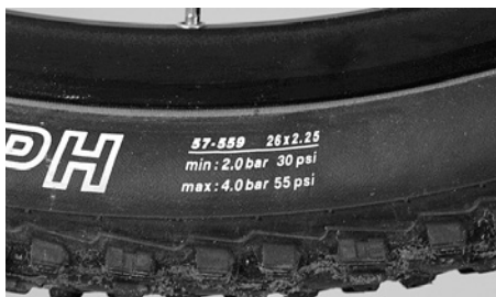
Air pressure range on the side of the tyre
