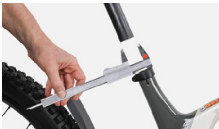
Make sure the seat post matches accurately the frame
