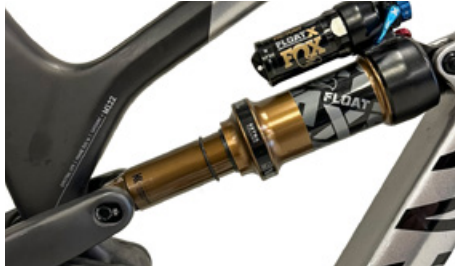
The O-ring displaced on the damper shows the spring travel used
