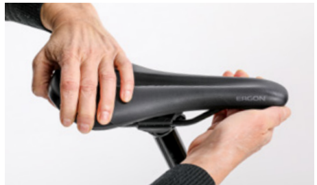
Trying to turn the saddle relative to the frame
