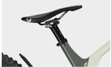
During freeriding etc. the saddle is normally tilted towards the rear
