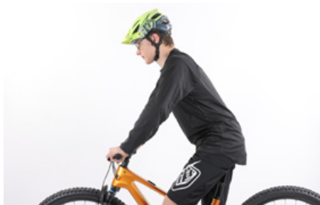
The inclination of your upper body is influenced by the distance between the grips of the handlebars and the saddle
