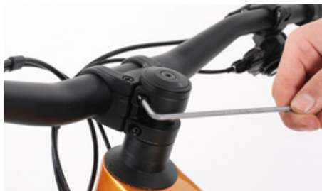
Loosen the bolts on the side of the stem
