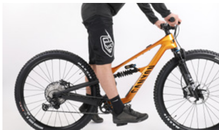
The leg must be fully stretched with the heel on the pedal at its lowest point
