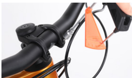
Retighten the bolts to the prescribed torque
