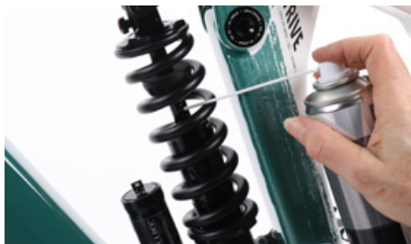
Apply some authorized lubricant after cleaning
