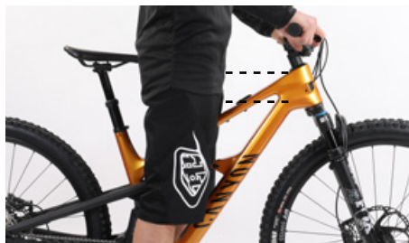
Be sure there is enough clearance between crotch and top tube
