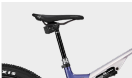
The upper edge of the saddle should remain as horizontal as possible
