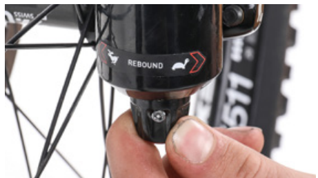
Rebound damping slows down the rebound
