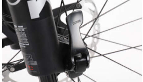
Make sure the quick-release lever is accurately closed
