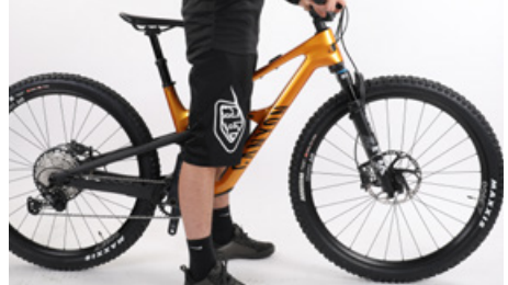
Checking the clearance between top tube and crotch
