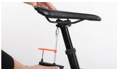
Retighten the bolts evenly and alternately to the prescribed torque value
