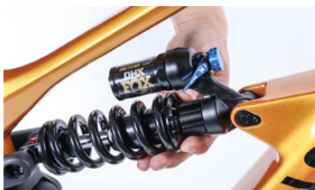
With steel coil springs the spring tension is altered with the knurled adjusting ring
