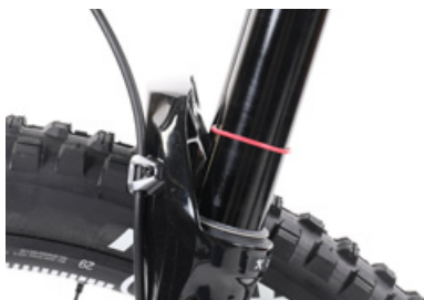
With the displaced cable binder you can find out the used spring travel
