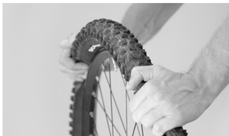
Press the tyre to both sides to make sure the inner tube does not get caught between rim and tyre beads
