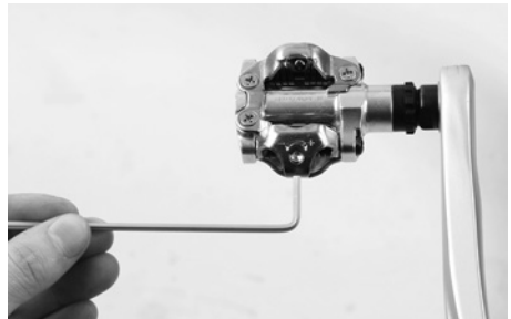
Adjust the required releasing force according to your needs
