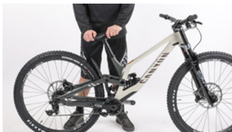
Press the saddle downwards
