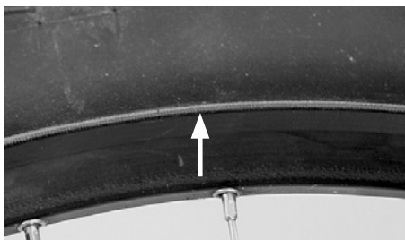
Witness line to check the correct seat of the tyre
