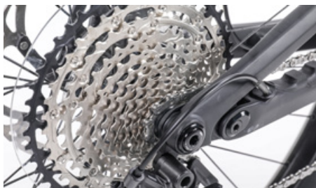
Store the bike with the chain on the smallest sprocket
