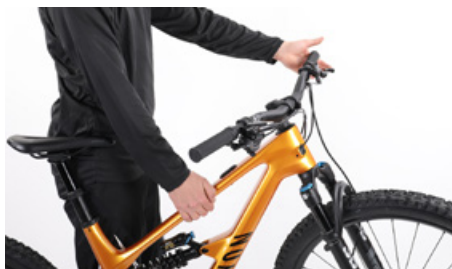
To check the bearing for ease of running, lift the front wheel and move it
