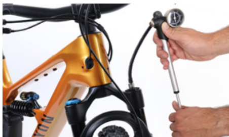
Adjusting the spring rate with a damper pump
