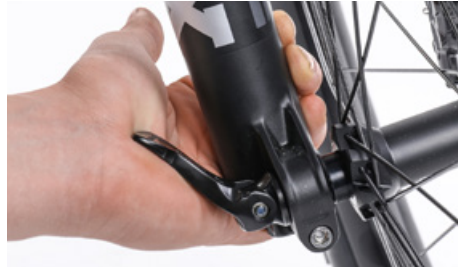
Closing the quick-release lever with the ball of your thumb
