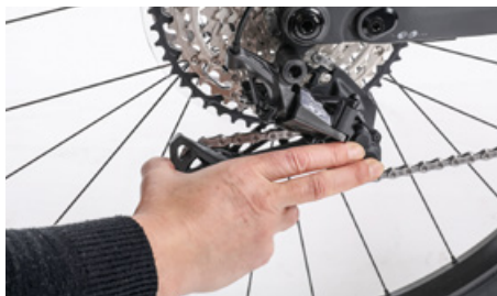
Check whether the rear derailleur can get caught in the spokes
