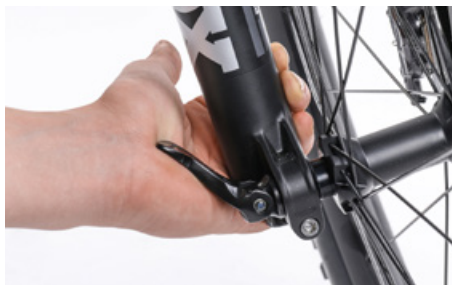
Check the reliable attachment of the wheels
