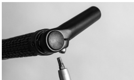
Retighten the bolts to the necessary torque value
