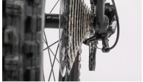
Look from the rear on the cassette sprockets and check, whether the pulleys of the rear derailleur are exactly under the cogs of the matching sprocket
