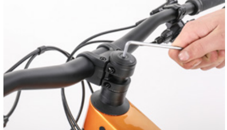
Adjust the bearing play by means of the countersunk adjusting bolt at the top after releasing the clamping bolts on the side
