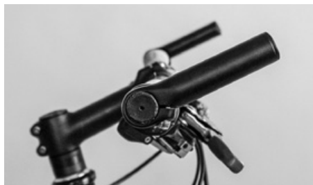
Bar ends give you additional ways of gripping the handlebar
