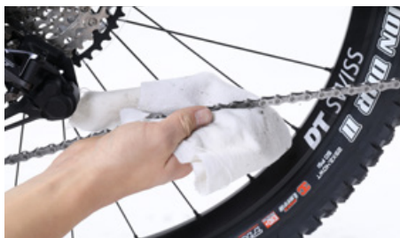
Clean the chain from dirt and oil with a rag
