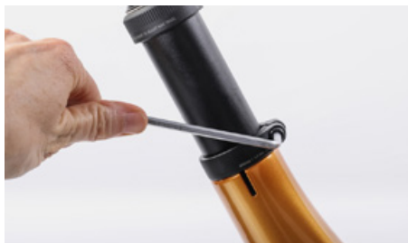
To adjust the saddle height loosen the saddle clamp
