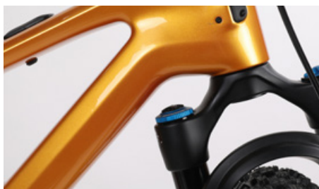
The fork crown must be freely rotatable without touching the frame
