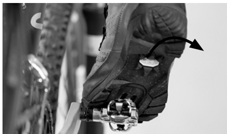
The clipless pedal disengages by an outward twisting of the heel
