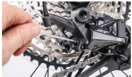
Reduce the swivel range of the rear derailleur with the limit screws
