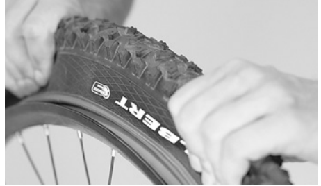
Press the tubeless tyre towards the centre of the rim
