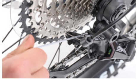
To adjust the clearance between pulley cage and sprocket, turn the bolt located at the front side of the drop-out
