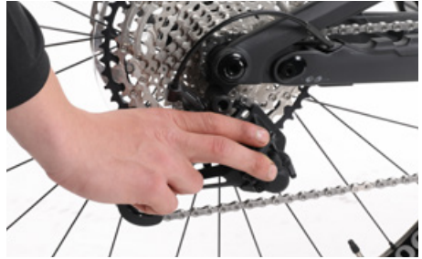
Check that the rear derailleur keeps clear of the spokes
