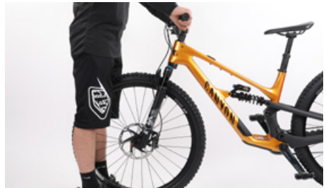
Try twisting the handlebars relative to the front wheel
