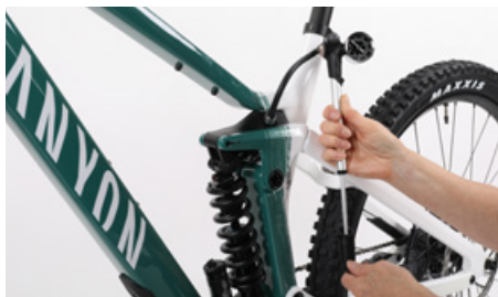
Air dampers are adjusted by modifying the air pressure
