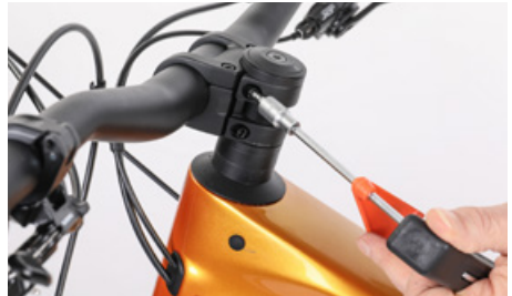
Retighten the clamping bolts located on the side of the stem by using a torque wrench
