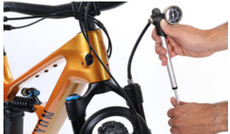
Check the air pressure of air suspension forks regularly
