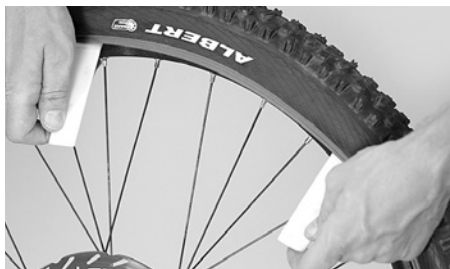
Apply the tyre levers and lift the tyre bead over the rim edge
