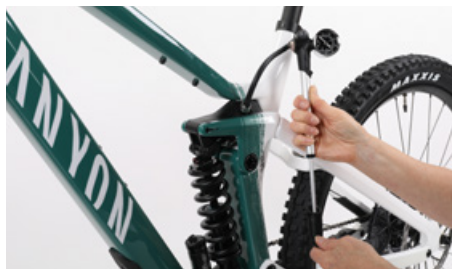
Check the air pressure of air suspension forks regularly
