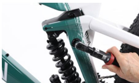
Check the tight fit of all rear frame screwings regularly according to the prescribed torque values
