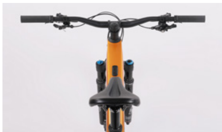
Check alignment of saddle along top tube to make sure it is not twisted
