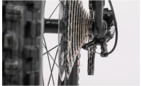
Shift to the smallest sprocket before removing the rear wheel
