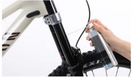
Apply some authorized lubricant after cleaning
