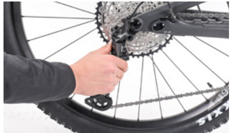
Pull the rear derailleur slightly to the rear to remove the rear wheel
