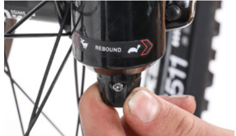
Adjustable rebound damping
