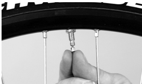
With race or Sclaverand valves the valve must be unscrewed
