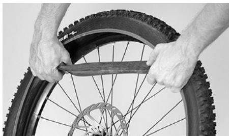
Remove the inner tube from the tyre
