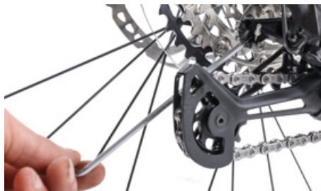
Retightening the Bowden cable at the rear derailleur: loosen the bolt that holds the Bowden cable tight first
