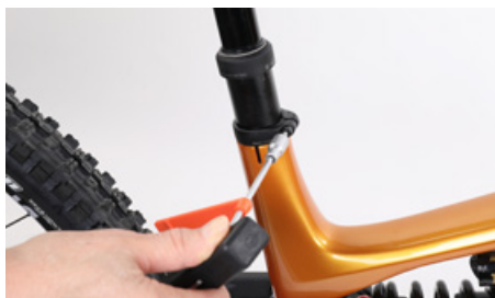
Observe the indicated torque value for the seat post clamp
