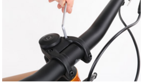
Release the bolts of the front plate of the stem
