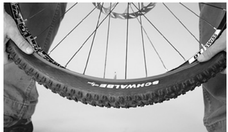
Press the tyre with your hand onto the rim
