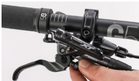
Adjusting the gripping distance of the brake lever
