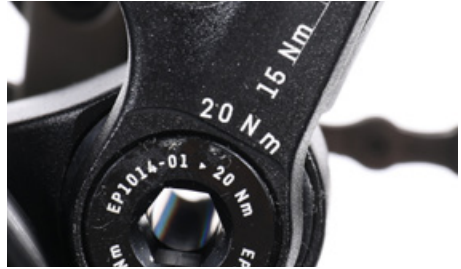
Always observe the tightening torques
