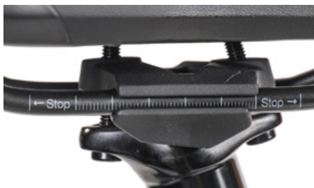
Be sure the saddle rail is clamped within the marked area
