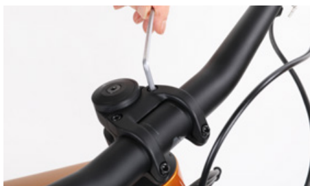
Release the Allen bolt(s) at the front side of the stem
