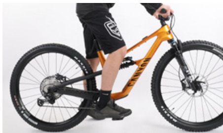
The ideal pedalling position: If the ball of your big toe is in the centre of the pedal, your knee should be slightly bent
