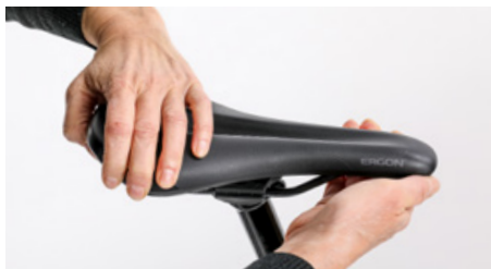
Try twisting the saddle relative to the frame
