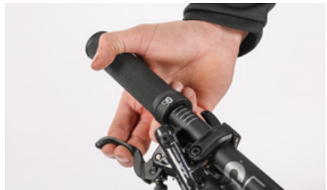
You should not be able to pull the brake lever all the way to the handlebars
