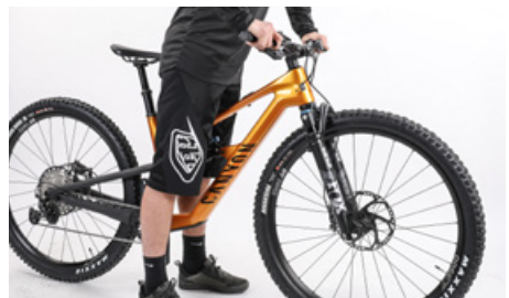
Compress the fork with the front wheel brake activated
