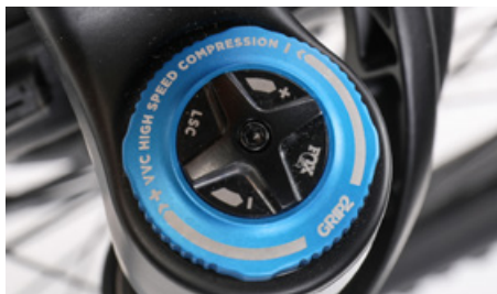
Compression damping slows down the compression
