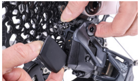
Remove the SRAM battery for charging
