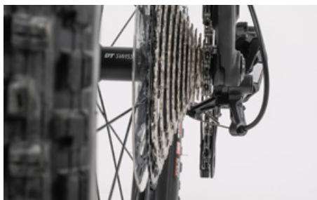
Look from the rear at the rear gear cluster and check whether the pulleys are perfectly aligned with the teeth of the adequate sprocket
