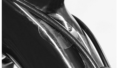
Special pads protect carbon from damage
