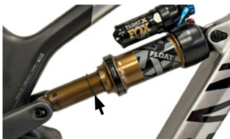
The O-ring displaced on the damper shows the spring travel used
