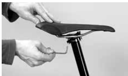
Release both bolts by 2 to 3 turns at the most
