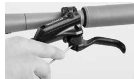
Adjusting the gripping distance of the brake lever
