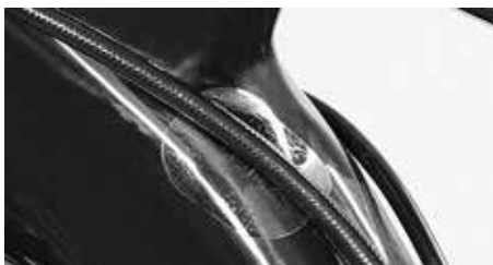
Special pads protect carbon from damage
