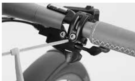
Tighten the brake and shift lever mounts to the prescribed torque values
