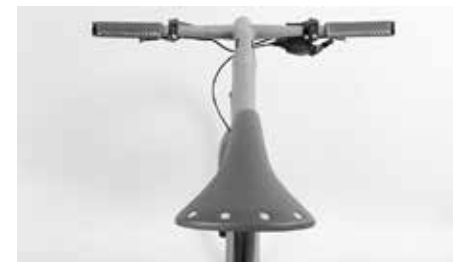
Check alignment of saddle along top tube to make sure it is not twisted
