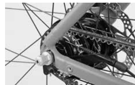
The belt drive transmits the force to the gear hub
