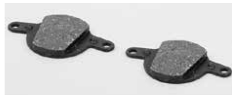
Brake pads with a width of less than a millimetre must be replaced with original spare parts
