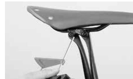
Tighten both bolts evenly and alternately without exceeding the permissible maximum torque value
