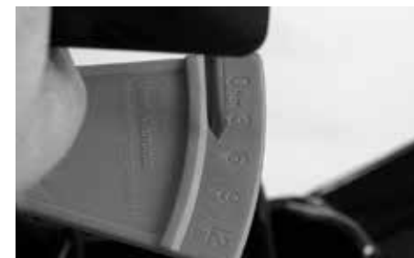
The pointer moves over the scale. Stop the turning movement as soon as the pointer reaches the number of the prescribed torque value.
