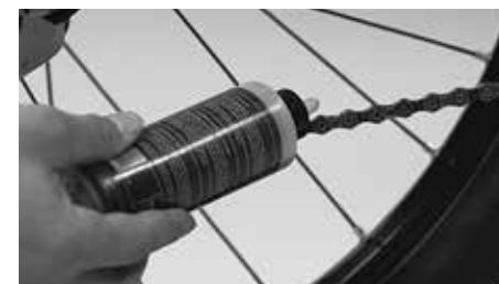
Finish cleaning your Canyon by lubricating the chain
