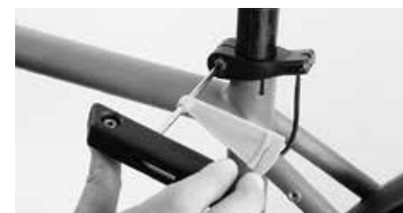
Tighten the lock nut by using the Canyon torque wrench according to the torque values on the component
