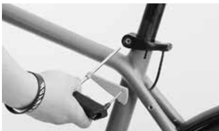
To adjust the height loosen the seat post binder bolt
