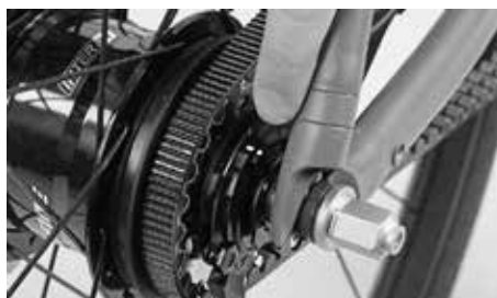
Make sure the belt runs properly over the rear belt wheel
