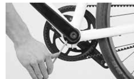
Turning the eccentric bearing, increasing tension
