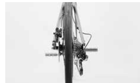
Look from the rear at the rear gear cluster and check whether the pulleys are perfectly aligned with the teeth of the adequate sprocket
