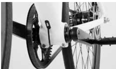
Check the proper fit of the eccentric bearing in the BB shell
