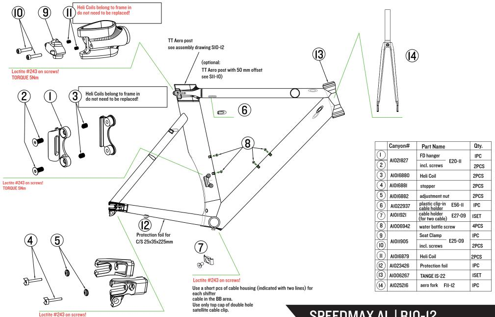
Note: Part 4 is assymetrical! Make it flush on inside and outside. SPEEDMAX AL | R10-12
