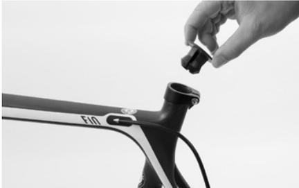
Remove the protective cap from the top end of the seat tube. Release the seat post binder bolt at the seat tube. Read beforehand chapter “Adjusting the Canyon road bike to the rider” in your bicycle manual Road bike and on the enclosed CD.
