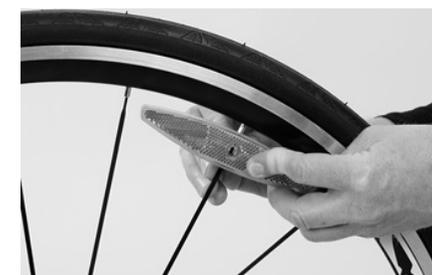
Finish by mounting the spoke reflectors. Make sure you mount two reflectors opposite of each other to the spokes of the front wheel and two reflectors opposite of each other to the spokes of the rear wheel.
