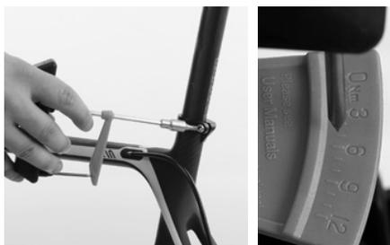
Slowly turn the handle of the Canyon Torque Wrench. Once the bolt is getting tight, the pointer moves over the scale. Stop the turning movement as soon as the pointer reaches the number for the specified torque.
