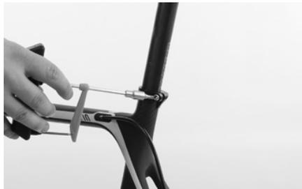
Bring the saddle into alignment and do not overtighten the seat post binder bolt, i.e. do not exceed the permissible maximum torque. Use the Canyon Torque Wrench.
