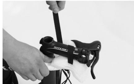
Keep hold of the handlebars and undo the band with Velcro fastener in the top at the stem fixing the handlebars.
