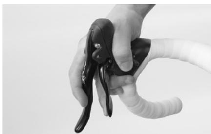
Check the proper functioning of the gears. Shift through all gears and make sure the rear derailleur does not collide with the spokes when the chain runs on the largest sprocket.
