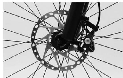
If you have disc brakes, check before mounting the wheel whether the brake pads rest snugly in their seats in the brake calliper. The gaps between the brake pads and the wheel should be parallel and the wear indicators in their correct position. Make sure you guide the rotor carefully between the brake pads.
