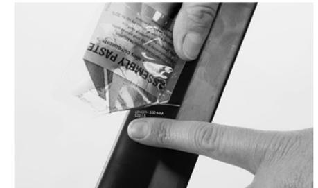
Apply a little Canyon assembly paste on the bottom part of the seat post and inside the seat tube.
