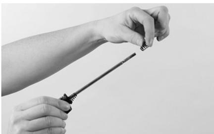
Take the quick-release for the front wheel out of the small parts box. Release the counternut and remove one of the springs from the quick-release.
