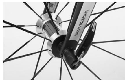
Check whether the front wheel is properly seated in the drop-outs and whether it runs accurately in the centre between the fork arms.
