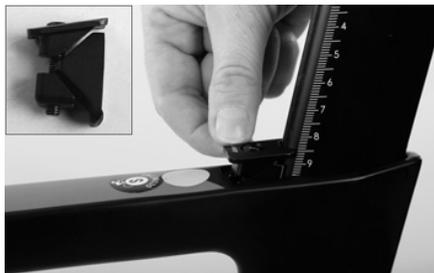
Slide the seat post into the seat tube to the desired saddle height. Insert the built-in seat post clamp.
