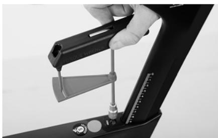
Tighten up the Allen bolt of the seat post clamp to the prescribed torque of 4 Nm up to a maximum of 6 Nm.
