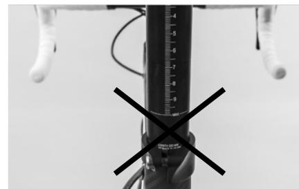
Your seat post must go into the frame as a minimum to as far as underneath the top tube and up to the MAX marking of the seat post.
