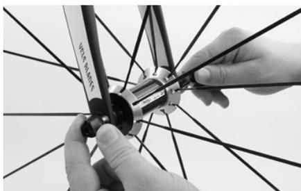
Tighten up the counter nut with the quick-release lever open until the quick-release lever builds up force when closed. Make sure the closed lever is close to the fork and does not stand out to the side or the front.
