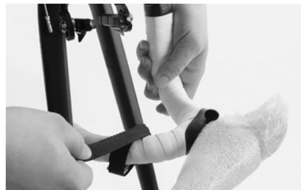
Keep hold of the handlebars to prevent any twisting, dropping and damage. Undo the band with Velcro fastener fixing the handlebars in the bottom to the fork.
