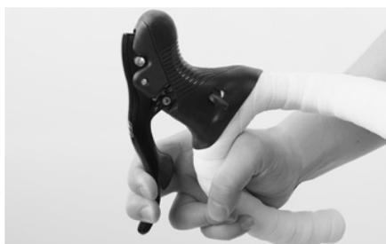
After mounting the wheel and tightening the quick-release pull the brake lever (several times, if you have disc brakes). Check the braking response of both brakes. It must be reached after the same travel and be stable at once.
