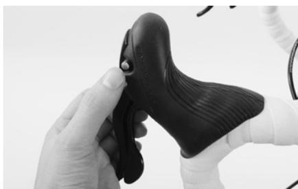
Re-close the release lever of the brake (Shimano, SRAM) immediately or move the bolt at the shift/brake lever back to its original position (Campagnolo) with the brake lever slightly activated.
