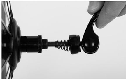
Make sure there is one spring on either side of the hub. When mounting the springs on either side of the quick-release, make sure their small-diameter ends face the hub. The quick-release lever is mounted to the left side, i.e. opposite the chain drive.
