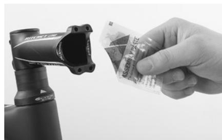
This is especially useful in the clamping areas of handlebars and stem, steerer tube and stem and seat post and stem, i.e. three areas where too much clamping force can damage either component, causing component failure or voiding the warranty. By reducing the clamping force, Canyon assembly paste relieves stress on sensitive carbon surfaces, preventing damage to fibres or the cracking of the carbon substructure.
