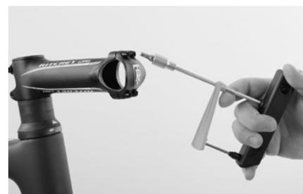
Put the matching bit into the holder of the Canyon Torque Wrench. Release the clamping bolts of the stem faceplate and remove the faceplate.
