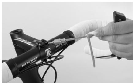
Use the Canyon Torque Wrench and finish by tightening the clamping bolts in cross pattern. Do not exceed the maximum tightening torques!
