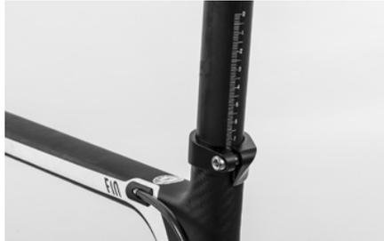
Slide the seat post into the seat tube to the desired saddle height.
