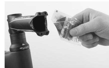
Open the Canyon assembly paste. Squeeze out some assembly paste and apply a thin layer of carbon assembly paste on the inner side of the faceplate as well as in the clamping area of the stem body.
