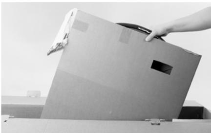
Remove the front wheel from the protective cardboard and from the wheel bag, if available.
