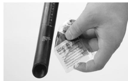
Prior to applying Canyon assembly paste, remove dirt particles and lubricant residues from the surfaces to be treated. Apply a thin and even film of Canyon assembly paste to the cleaned surfaces using a brush or a chamois. Mount the components, as specified. Use the Canyon Torque Wrench and never exceed the prescribed maximum tightening torque! Remove excessive Canyon assembly paste and re-seal the small sachet after use.
