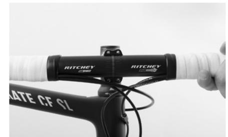
Position the handlebars by means of the marking accurately centred in the stem clamp. Make sure the bowden cables and the lines are not twisted or bent, but run in a smooth curve to the cable stops or brakes.
