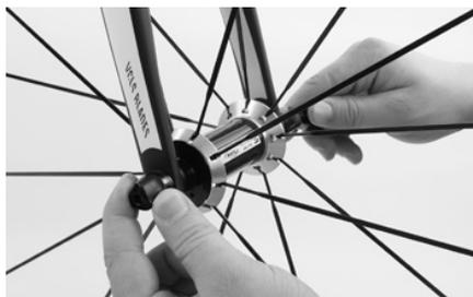
Tighten the counternut of the quick-release by no more than two full turns. Read up on quick-releases in chapter “**How to use the quick-release**” in your bicycle manual Road bike; also observe the instructions of the component manufacturers on the enclosed CD.
