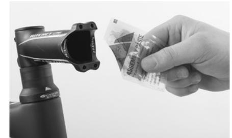
Open the Canyon assembly paste. Squeeze out some assembly paste and apply a thin layer of carbon assembly paste on the inner side of the faceplate as well as in the clamping area of the stem body.
