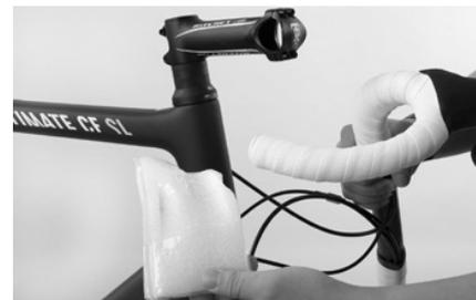
Remove the protective film and sleeves from the handlebars. It is recommended that you remove the protective material in general by hand. If that is not possible, it is best to use scissors, and if it is really necessary, use a box cutter.
