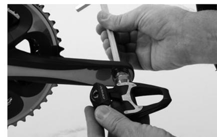
Screw each pedal manually into the thread of its crank by two to three full turns. Continue by using a pedal spanner to tighten the pedals firmly. Some pedal types have to be tightened with an Allen key.
