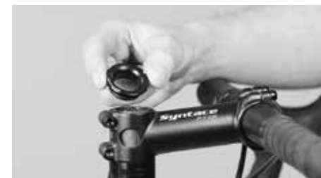
Retire a tampa terminal
