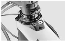
Some Canyon models with carbon frame are fitted with an Impact Protection Unit or IPU, which is an end stop. This IPU prevents the handlebars or its fittings from touching the top tube.
