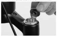
Before transport the suspension fork was completely deflated. The suspension fork has to be filled with the proper air pressure.
