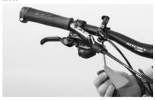
The brake lever and the shift lever are mounted to the handlebars. Mount the control lever to the handlebars on the inner side of the brake and shift lever clamps. Screw the bolt without tightening it, so that the control lever can still be turned and shifted.
