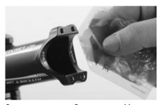
Squeeze out some Canyon assembly paste and apply a thin layer of carbon assembly paste on the inner side of the faceplate as well as in the clamping area of the stem body.
