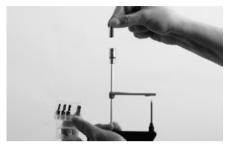
Put the matching bit into the holder of the Canyon Torque Wrench.
