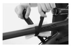
Keep hold of the handlebars and undo the band with Velcro fastener in the top area at the frame.
