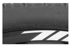
Inflate both tyres to the maximum pressure indicated on the side of the tyres. You can find more information on tyres and inner tubes in chapter "The wheels - tyres, inner tubes and air pressure" in your bicycle manual Mountain bike on the enclosed CD.
