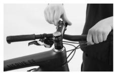
Turn the stem including fork towards the front, i.e. in direction of motion. Make sure the cables and lines are not twisted.
