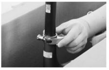
Bring the saddle into alignment and close the quick-release or the seat post binder bolt. Take care not to overtighten the seat post binder bolt or quick-release. Remove the protective film from the saddle, if available,
