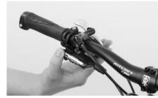
Release the bolt of the adjacent brake lever clamp and turn the brake lever downwards.
