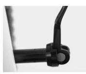
Make sure the quick-release lever is completely open and lies in the axle recess. As soon as the axle thread engages with the thread of the left fork leg, close the axle by turning it clockwise. During the first rotations you should be able to rotate the thru axle nearly without resistance.
