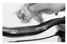
Prior to applying Canyon assembly paste, remove dirt particles and lubricant residues from the surfaces to be treated. Apply a thin and even film of Canyon assembly paste to the cleaned surfaces using a brush or a chamois.
