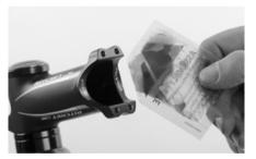
This is especially useful in the clamping areas of handlebars and stem, steerer tube and stem and seat post and seat tube, i.e. three areas where too much clamping force can damage either component, causing component failure or voiding the warranty.
