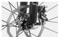
The rotor must not drag heavily on the brake calliper and normally not on the brake pads. Spin both wheels to make sure they run true.
