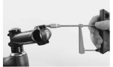
Take the Canyon Torque Wrench and put the bit matching the faceplate bolts into the holder.
