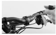
Position the faceplate on the handlebars. Retighten the clamping bolts of the faceplate evenly in a cross pattern until they lightly hold the handlebars in place.
