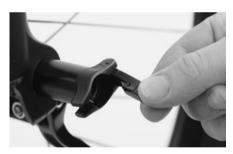
Bring the front wheel into the right position between the drop-outs and slide the axle from the right side through the drop-out and the hub. Unfold the lever from the axle.
