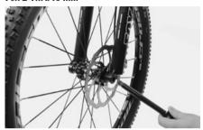
Put the front wheel into the fork and mount the rotor at the same time in the brake calliper. Bring the front wheel into the right position between the drop-outs and slide the axle with open E-Thru quick-release lever from the left side through the drop-out and the hub.
