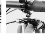
Assemble the shift lever to the Matchmaker. Tighten the bolt to the tightening torque of 2.8-3.4 Nm specified by SRAM.
