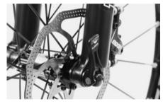
If the lever cannot be closed completely, reopen it and turn the axle a little anticlockwise. Try closing the quick-release lever once again.
