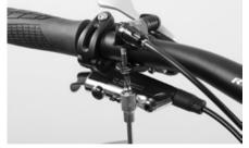
Now you can tighten the bolt of the control lever with the Canyon Torque Wrench.
