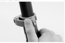
Measure the saddle height of your previous bicycle from the middle of the bottom bracket up to the top edge of the saddle in the middle of the saddle. Then transfer the saddle height to your new Canyon.
