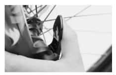
Close both quick-release levers. From the start of the closing movement up to about the first half of its travel the levers should move very easily without clamping the wheel, whereas over the second half of its travel the force you need to move it should increase considerably. Towards the end of its travel you should clearly feel resistance.
