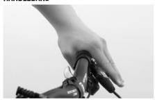
Make the adjustments of the handlebars with the front wheel mounted and the tyre inflated to the suitable pressure. The brake levers of a readyfor-use mountain bike point slightly downwards. When you sit in the saddle with your fingers on the brake levers the back of your hands should form a straight line with your forearms.
