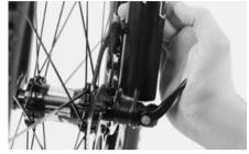
Close the E-Thru quick-release lever like a usual quick-release lever.
