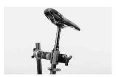
Do not clamp a frame tube or a carbon seat post of your Canyon in the holding jaws of the workstand! Use a suitable aluminium seat post for clamping instead. If you have a height-adjustable seat post, do not clamp the bike on a movable part, but only on the bottom part which is removed far enough. When inserting or pulling out the height-adjustable seat post, make sure to pull in or out the cable where it comes out of the frame to prevent any breaking of the cable.
