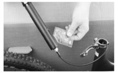
Make it a rule to use assembly paste on seat posts of mountain bikes to achieve a firm seat of the seat posts. Lowering the seat post during off-road use scratches the surface a little. This is normal wear and no reason for complaint.
