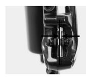
If your Canyon has disc brakes, check before mounting the wheel whether the brake pads rest snugly in their seats in the brake calliper body. This is the case when the gap between the brake pads is parallel.
