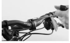
Use the Canyon Torque Wrench and finish by tightening the clamping bolts in cross pattern. Do not exceed the maximum tightening torques mainly printed on the stem!
