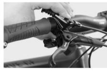
The shift lever is mounted to the handlebars, the brake lever however not.
