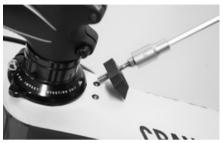
Make sure the stem including handlebars shows in direction of motion. Position the IPU on the top tube with the rounded side pointing in direction of motion and the bevelled part to the rear levelling off with the top tube.
