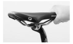
Bring the saddle into alignment and do not overtighten the quick-release or the seat post binder bolt, i.e. do not exceed the permissible maximum torque. Use the Canvon Torque Wrench.
