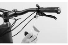
Tighten the bolt to the tightening torque of 5-6 Nm specified by SRAM.
