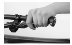
After the wheel mounting do a brake test when stationary. Actuating the brake lever should generate a clear-cut braking response before the lever touches the handlebars. You can find further information in chapter "The brake system" in your bicycle manual Mountain bike on the enclosed CD.
