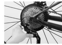
Check the proper functioning of the gears. Shift through all gears and make sure the rear derailleur does not collide with the spokes when the chain runs on the largest sprocket.
