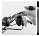
Slowly turn the handle of the Canyon Torque Wrench. Once the bolt is getting tight, the pointer moves over the scale. Stop the turning movement as soon as the pointer reaches the number for the specified torque.
