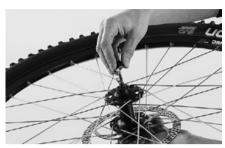
Tighten the counternut of the quick-release by no more than two full turns. Read up on quick-releases in chapter "How to use the quick-releases and thru axles" in your bicycle manual Mountain bike; also observe the instructions of the component manufacturers on the enclosed CD.
