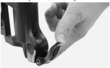
The 20-mm thru axle system provides several appliances to fix the front wheel. To mount the front wheel open both quick-release levers in the bottom area of both fork legs. Put the front wheel into the fork and mount the rotor at the same time in the brake calliper.
