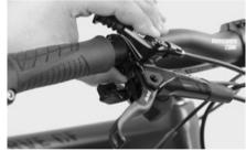
Remove the protective film from the right brake lever.
