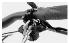
Bring the brake lever in the same position as the left brake lever assembled by the manufacturer. Tighten the bolt to the tightening torque of 5-6 Nm specified by SRAM.
