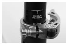
Your seat post must go into the frame as a minimum to as far as underneath the top tube and up to the MIN/MAX marking of the seat post.
