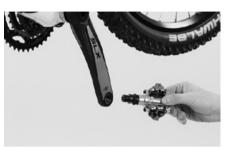
Screw each pedal manually into the thread of its crank by two to three full turns. Continue by using a pedal spanner to tighten the pedals firmly.
