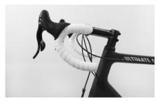
Verify that the upper grip areas of the shift/ brake levers are in horizontal position. The ends of the drops are then in parallel to the ground or point slightly downwards.
