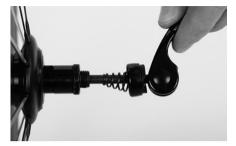
Make sure there is one spring on either side of the hub. When mounting the springs on either side of the quick-release, make sure their small-diameter ends face the hub. The quick-release lever is mounted to the left side, i.e. opposite the chain drive.
