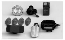
Fix the white reflector to the handlebars and the red reflector to the seat post, the spoke reflectors as well as a bell.
