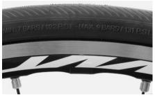
Inflate both tyres to the maximum pressure indicated on the side of the tyres. You can find more information on tyres and inner tubes in chapter "The wheels - tyres, inner tubes and air pressure" in your bicycle manual Road bike on the enclosed CD. Finish the assembly by carrying out thoroughly the tests described in chapter "Before your first ride".
