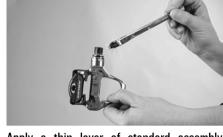
Apply a thin layer of standard assembly grease on the pedal threads before screwing in the pedals.
