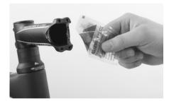
This is especially useful in the clamping areas of handlebars and stem, steerer tube and stem and seat post and stem, i.e. three areas where too much clamping force can damage either component, causing component failure or voiding the warranty. By reducing the clamping force, Canyon assembly paste relieves stress on sensitive carbon surfaces, preventing damage to fibres or the cracking of the carbon substructure.
