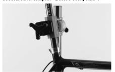
Do not clamp a frame tube or a carbon seat post of your Canyon in the holding jaws of the workstand! Be sure to only use a suitable aluminium seat post for clamping. It is best to use a workstand that holds the frame from inside at three points or else ask someone to help while you assemble your bike.
