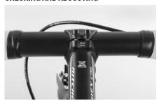
Make sure the upper and lower clamping slots between faceplate and stem body are parallel and identical in width. Release the clamping bolts, if necessary, and re-tighten them slightly and evenly.
