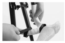
Keep hold of the handlebars to prevent any twisting, dropping and damage. Undo the band with Velcro fastener fixing the handlebars in the bottom to the fork.
