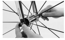
Tighten the counternut of the quick-release by no more than two full turns. Read up on quick-releases in chapter "How to use the quick-release" in your bicycle manual Road bike; also observe the instructions of the component manufacturers on the enclosed CD.
