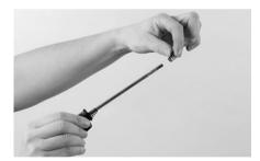
Take the quick-release for the front wheel out of the small parts box. Release the counternut and remove one of the springs from the quick-release.
