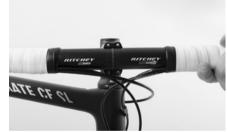
Retighten the clamping bolts of the faceplate evenly in a cross pattern until they lightly hold the handlebars in place.
