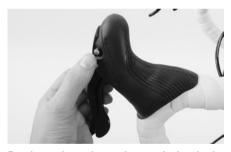
Re-close the release lever of the brake (Shimano, SRAM) immediately or move the bolt at the shift/brake lever back to its original position (Campagnolo) with the brake lever slightly activated.
