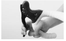
After mounting the wheel and tightening the quick-release pull the brake lever (several times, if you have disc brakes). Check the braking response of both brakes. It must be reached after the same travel and be stable at once.
