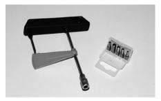
We regard the use of a torque wrench as essential so as to ensure the two parts can be fixed together securely and safely.
