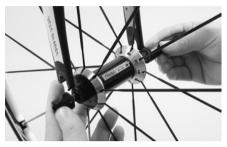
Mount the front wheel by sliding the hub together with the quick-release into the dropouts.
