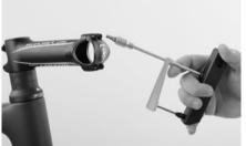
Put the matching bit into the holder of the Canyon Torque Wrench. Release the clamping bolts of the stem faceplate and remove the faceplate.
