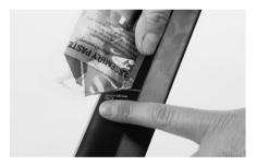
Apply a little Canyon assembly paste on the bottom part of the seat post and inside the seat tube.
