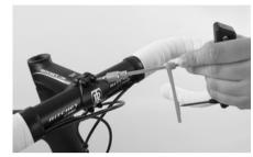
Use the Canyon Torque Wrench and finish by tightening the clamping bolts in cross pattern. Do not exceed the maximum tightening torques!
