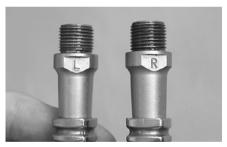
Before mounting the pedals, check the marking on the pedal axles first. "R" stands for right pedal and "L" for left pedal. Note that the left pedal has a left-handed thread that has to be tightened contrary to the direction you are accustomed to, i.e. anticlockwise.
