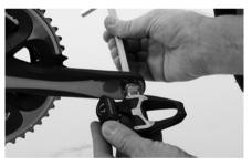
Screw each pedal manually into the thread of its crank by two to three full turns. Continue by using a pedal spanner to tighten the pedals firmly. Some pedal types have to be tightened with an Allen key.
