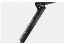
Some Canyon models (e.g. Speedmax CF and Speedmax AL) have an oval shaped seat post. Mounting anything than the standard seat post is therefore impossible. Release both Allen bolts at the seat post clamp.
