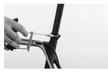
Bring the saddle into alignment and do not overtighten the seat post binder bolt, i.e. do not exceed the permissible maximum torque. Use the Canvon Torque Wrench.
