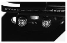
Exceeding the maximum torque at the clamping bolts (e.g. at the stem, steerer tube, handlebars or seat post) leads to an excessively high clamping force. This can cause the component to fail and hence there is a high associated risk of accidents. In addition, the product guarantee would be null and void in such a case. Screws or bolts that are too loose or are done up too tightly can cause a failure and hence lead to an accident. Always follow exactly the tightening torque details from Canyon.
