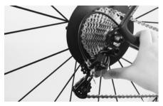
Shift through all gears and make sure the rear derailleur does not collide with the spokes when the chain runs on the largest sprocket.
