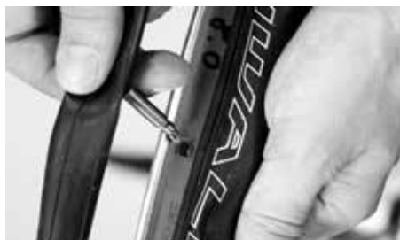
Sett ventilen i felghullet
